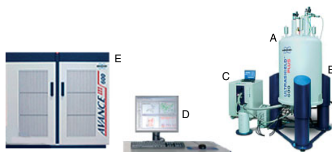
Figure 1 Modern NMR spectrometer: A, actively shielded superconducting magnet; B, antivibration posts; C, cryogenic cooling unit; D, primary computer; E, spectrometer console.
